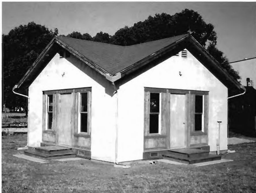
Figure 1. Villa Termiti used to test fumigation techniques and alternatives to fumigation for control of drywood termites. The Villa Termiti is symmetrical with all four sides structurally identical.
